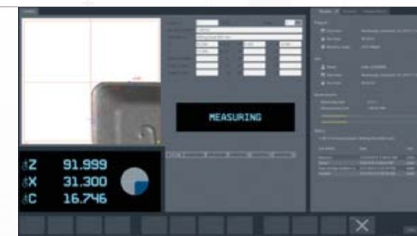
Cutting edge inspection in the »metis« tool analysis software
